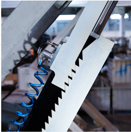
MECHANICAL SAFETY rack on cylinder with cold galvanizing treatment
