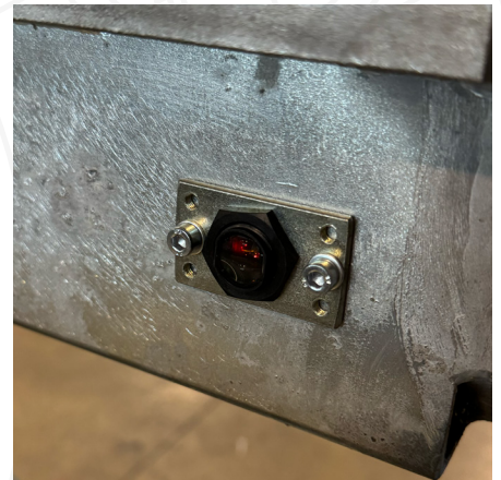
PHOTOCELLS detect any desynchronizations and immediately stop the lift
