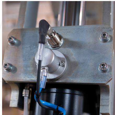
SECURITY STATUS SENSOR on mechanical safety rack
