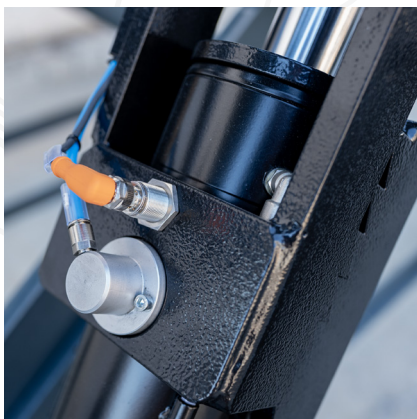
SECURITY STATUS SENSOR on mechanical safety rack
